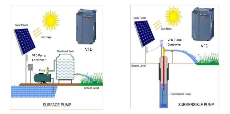
A typical solar water pumping system is known by the sum total of solar array size that is required to run the attached pump. A 1000 Wp solar water pump is capable of drawing and pumping approximately 40,000 liters of water per day from a source that is up to 10 meters deep. This is sufficient to irrigate about 2 acres of land with regular crops. A 1000 Wp solar water pump helps save up to Rs. 45,000 when compared to equivalent use of a diesel-operated pump over a year.
